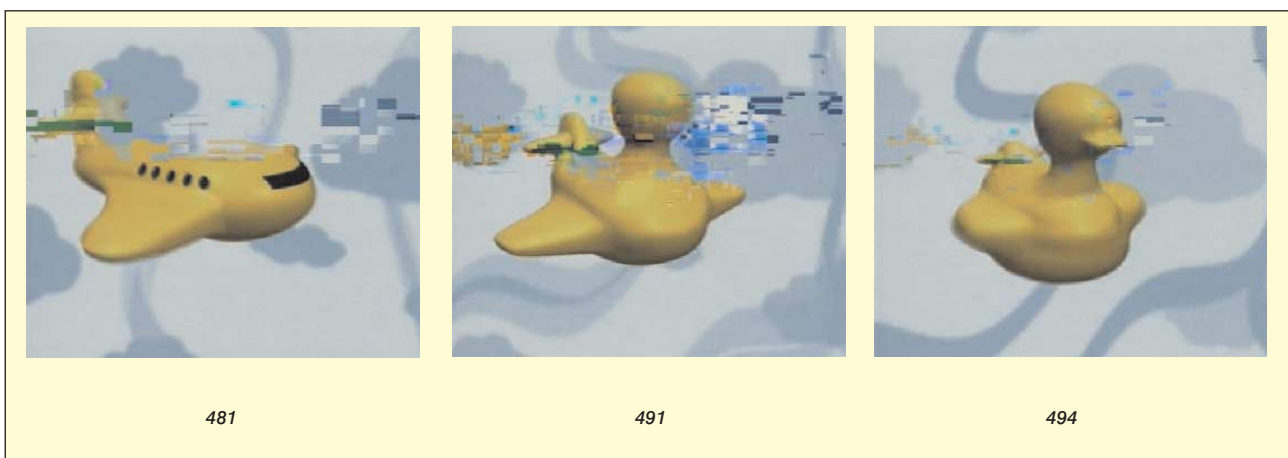
Fig. 8 Examples from frames 478–494. Blocking and tiling* errors span 17 frames.
