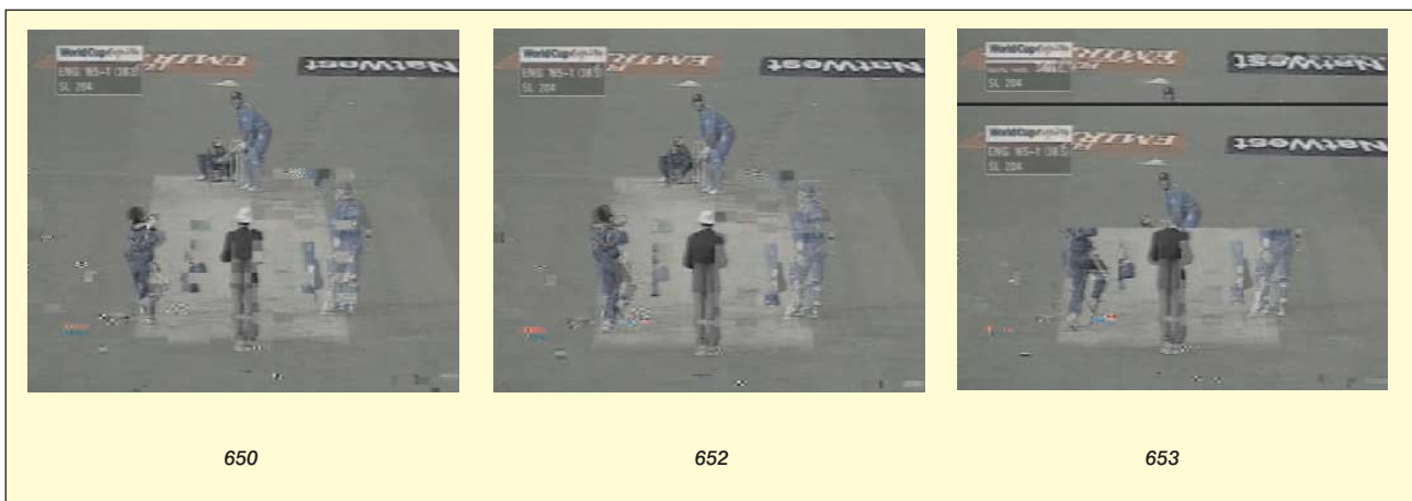
Fig. 9 Frames 650-653 contain a significant glitch. Full screen tiling is observable and a 'synchronisation' error occurs on frame 653.
